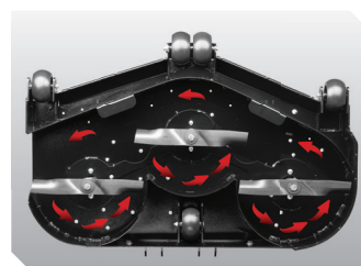
48", 54", and 60" Decks – Deep 7 gauge shell to tackle deep grass with ease
