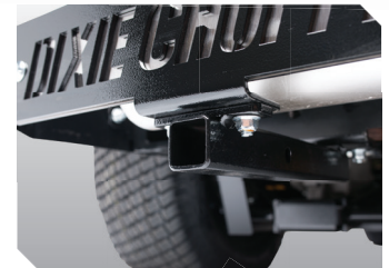
Hitch Receiver – Class 1 hitch for easier mounting of accessories
